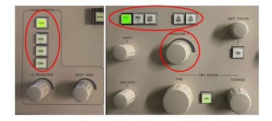
3. Press STD focus (right panel) and make sure OL current is 4.31 (CRT at right side of column).
