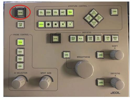
2. Make sure the operation mode is TEM MAG mode. Decrease mag using MAG/CAM L button and move sample around if cannot see beam. You can even change to LOW MAG mode to find the sample.
