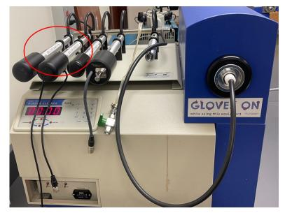
2. Put holder on sample loading station, with appropriate holder support lying underneath hold tip.
