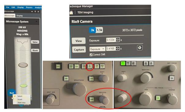
12. Objective/HC aperture: press OL/HC to insert high-contrast aperture to enhance contrast if needed.
