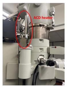
b. Pull out the ACD&Bake page (TEMCON---Maintenance---ACD&Bake) and enable ACD heat.
