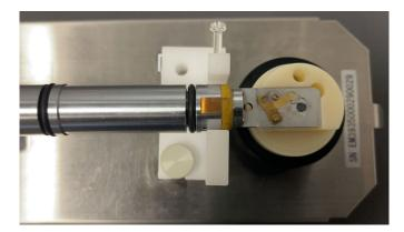
For double tilt holder, loosen two screws TWO turns, rotate the two plate-clamping fingers and mount sample facing DOWN.
