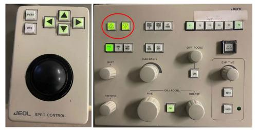
6. Correct condenser stigmatism: press COND STIG and adjust DEF-X & DEF-Y knobs to make beam round.
