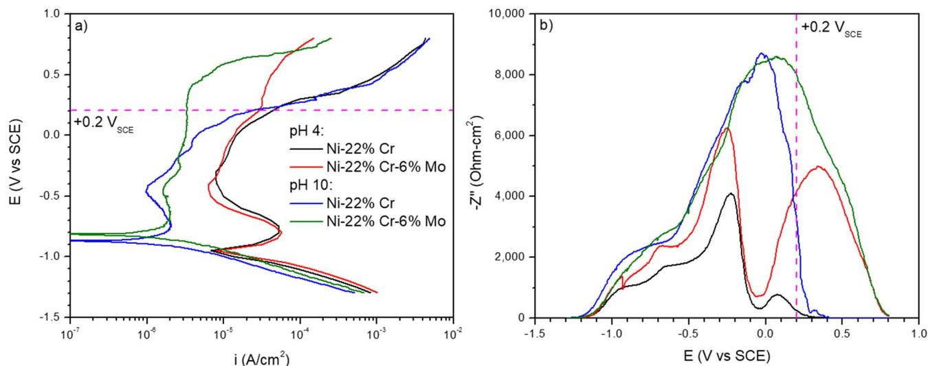
**Figure 4.** a) Current density and b) impedance variations during upward potentiodynamic polarization of Ni-22 Cr and Ni-22 Cr-6 Mo, wt%, in deaerated 0.1 M NaCl at pH 4 and 10 with the potential used in this study (+0.2 V<sub>SCE</sub>) indicated.
