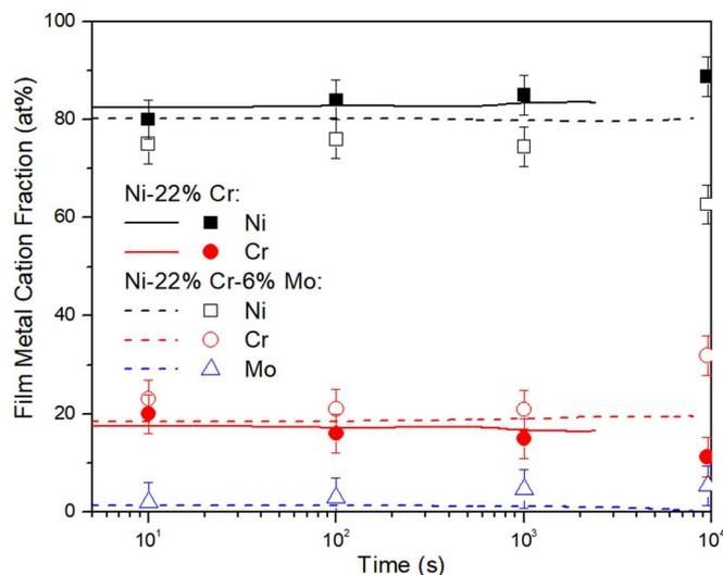
**Figure 10.** Relative accumulation of metal cations in the passive films during growth until the time of localized corrosion initiation at  $+0.2 V_{SCE}$  according to ICP-MS (lines) and XPS (symbols) measurements on Ni-22 Cr and Ni-22 Cr-6 Mo, wt%, in 0.1 M NaCl pH 10.
