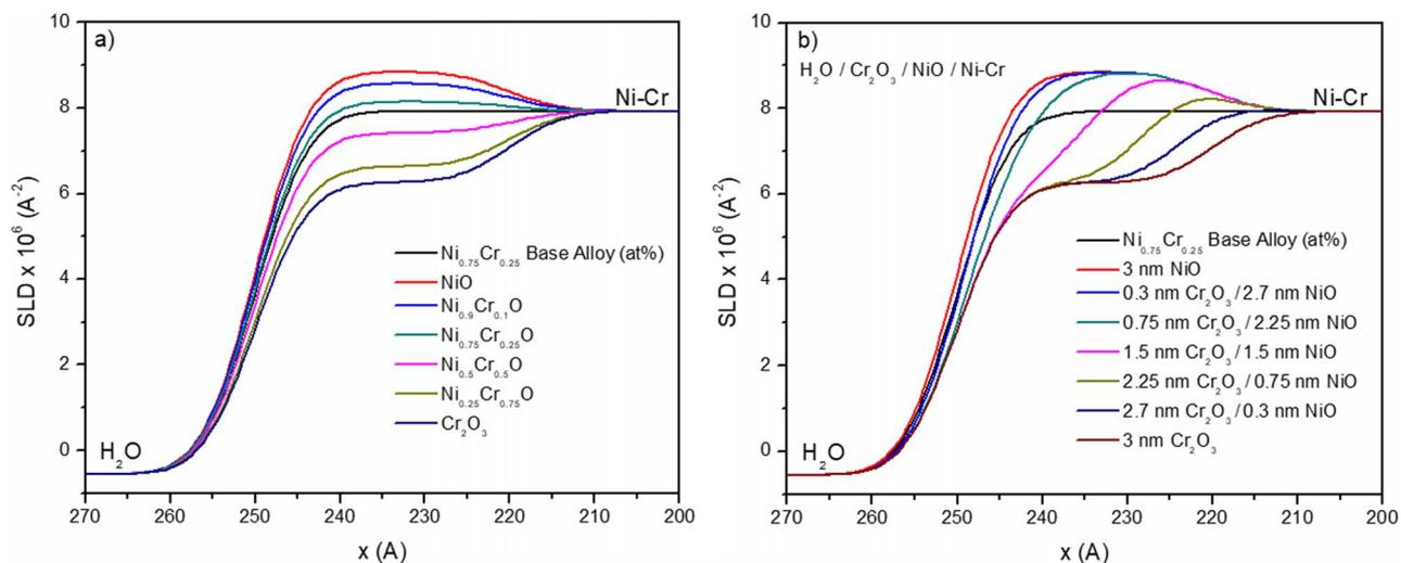
**Figure 14.** Simulated SLD profiles for a) a solute-captured rocksalt-structured oxide,  $\text{Ni}_{1-x}\text{Cr}_x\text{Cr}_2\text{O}_4$  containing varying %  $\text{Cr}^{3+}$  and b) a bilayer oxide comprised of  $\text{Cr}_2\text{O}_3$  and NiO with varying thicknesses of each conformal layer. An interfacial roughness of 5 Å was used to replicate the experimental parameters.
