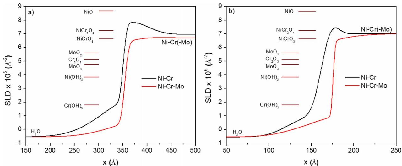
**Figure 13.** SLD profiles obtained for deposited Ni-20% Cr and Ni-20% Cr-10% Mo, wt%, films passivated up to +0.2 V<sub>SCE</sub> in a) 0.1 M NaCl pH 4 and b) 0.1 M NaCl pH 10 solutions with the theoretical SLD for various possible compounds shown to indicate their presence and distribution through the films.
