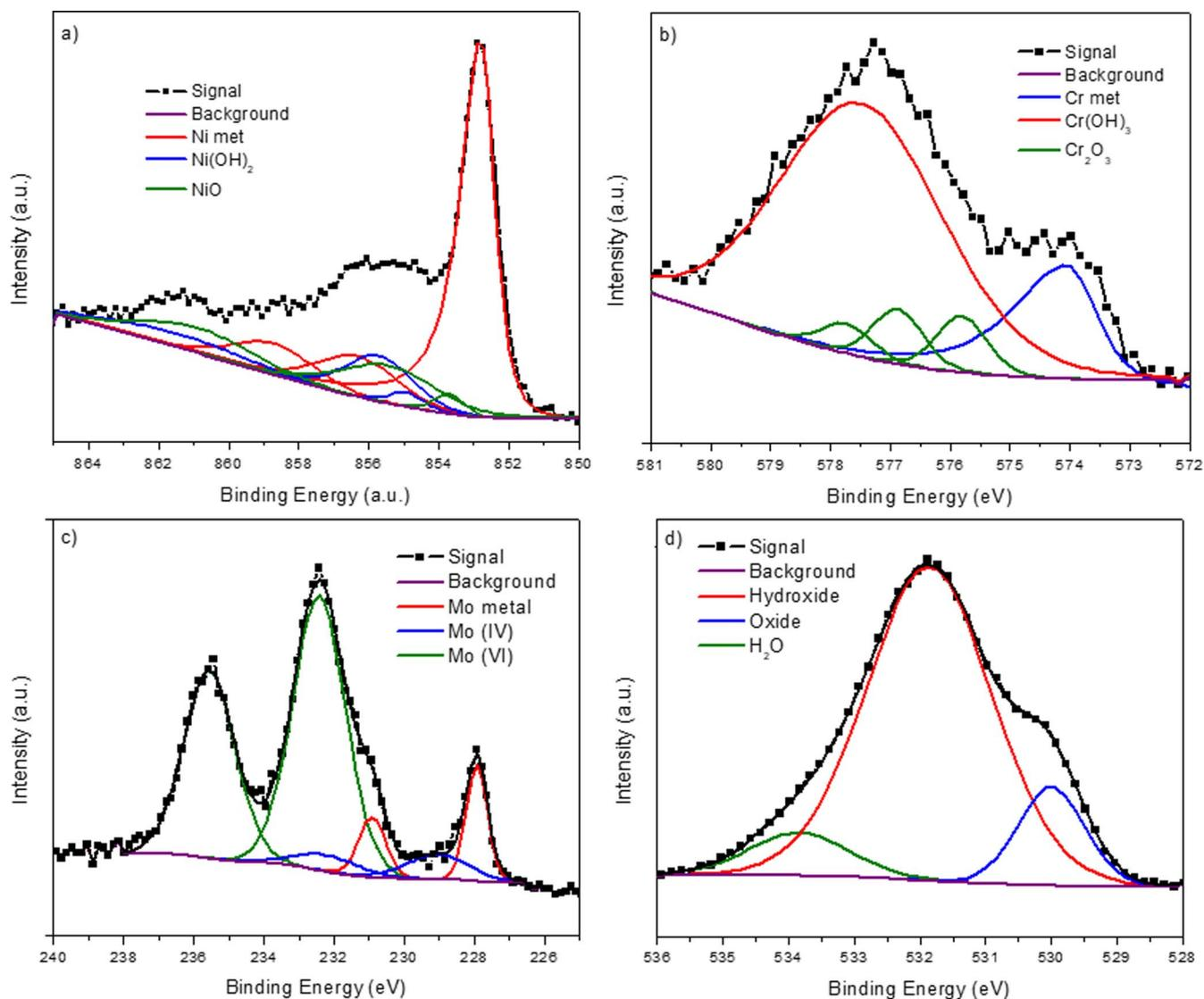
**Figure 11.** De-convoluted XPS spectra for a) Ni 2p<sup>3/2</sup>, b) Cr 2p<sup>3/2</sup>, c) Mo 3d, and d) O 1s bands collected on Ni-22 Cr-6 Mo, wt%, passivated at +0.2 V<sub>SCE</sub> for 10 ks in 0.1 M NaCl pH 4.
