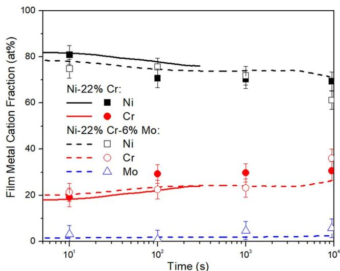
**Figure 7.** Relative accumulation of metal cations in the passive films during oxide growth until the time of localized corrosion initiation at  $+0.2 V_{SCE}$  according to ICP-MS (lines) and XPS (symbols) measurements on Ni-22 Cr and Ni-22 Cr-6 Mo, wt%, in 0.1 M NaCl pH 4.
