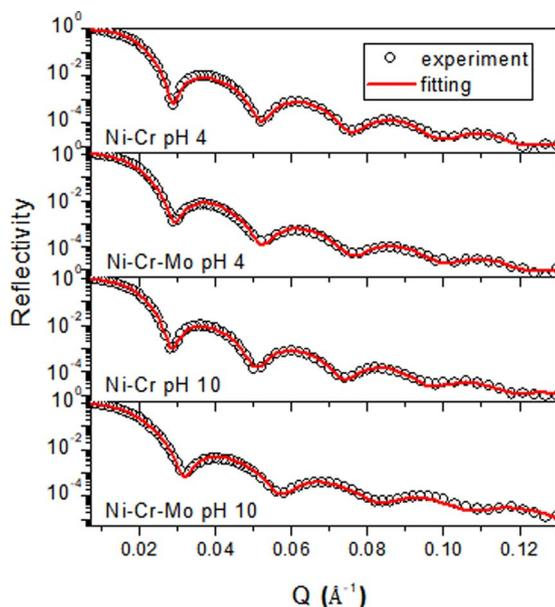
**Figure 12.** In-situ neutron reflectometry data collected during potentiostatic experiments and the fitted reflectivity curves for deposited Ni-20% Cr and Ni-20% Cr-10% Mo, wt%, films exposed to 0.1 M NaCl pH 4 and pH 10 solution.
