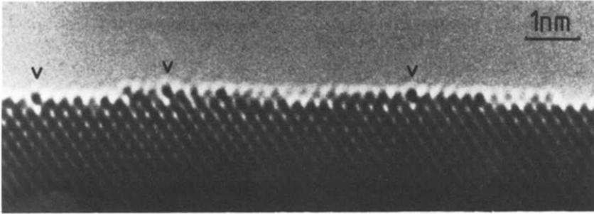
Fig. 1. High resolution electron micrograph of an extensive area of gold (100)  $1 \times 1$  surface with surface defects arrowed. The small normal displacements can best be seen by viewing along the surface from one side.
