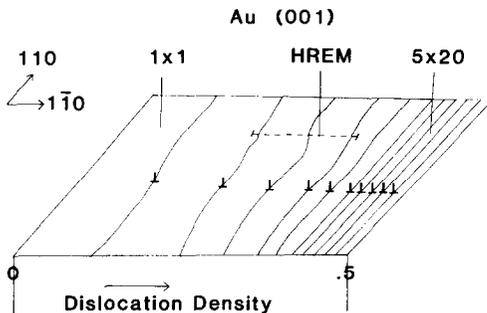
Fig. 3. Schematic diagram of the gold (100) surface in terms of surface dislocations. To the left, the pure  $1 \times 1$  surface contains no dislocations whilst the  $5 \times 20$  hexagonal reconstruction can be represented as a 50% dislocation coverage. The experimentally observed surfaces are between the two extremes as indicated.
