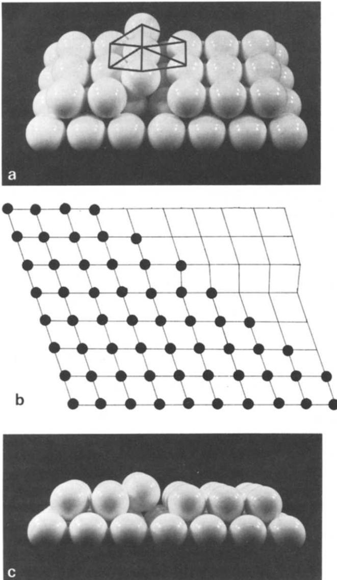
Fig. 2. The proposed Shockley partial dislocation structure in (a) sphere model at an angle, (b) in terms of a cut bulk partial dislocation and (c) the sphere model viewed along the electron beam direction. The pseudo-hexagonal core structure of the dislocation is indicated in (a). In (b), the large discs correspond to the atomic columns retained after the surface cut.
