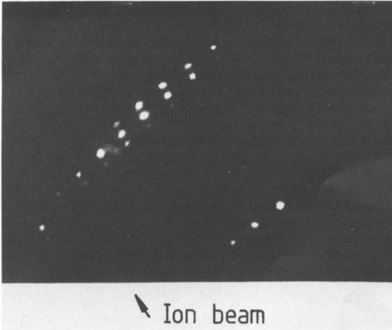
Fig. 4. LEED diffraction pattern of the reconstructed Pt(100) surface following ion bombardment at a grazing angle along [011], courtesy of R.C. Stair [10]. Only one domain of the reconstruction occurs.
