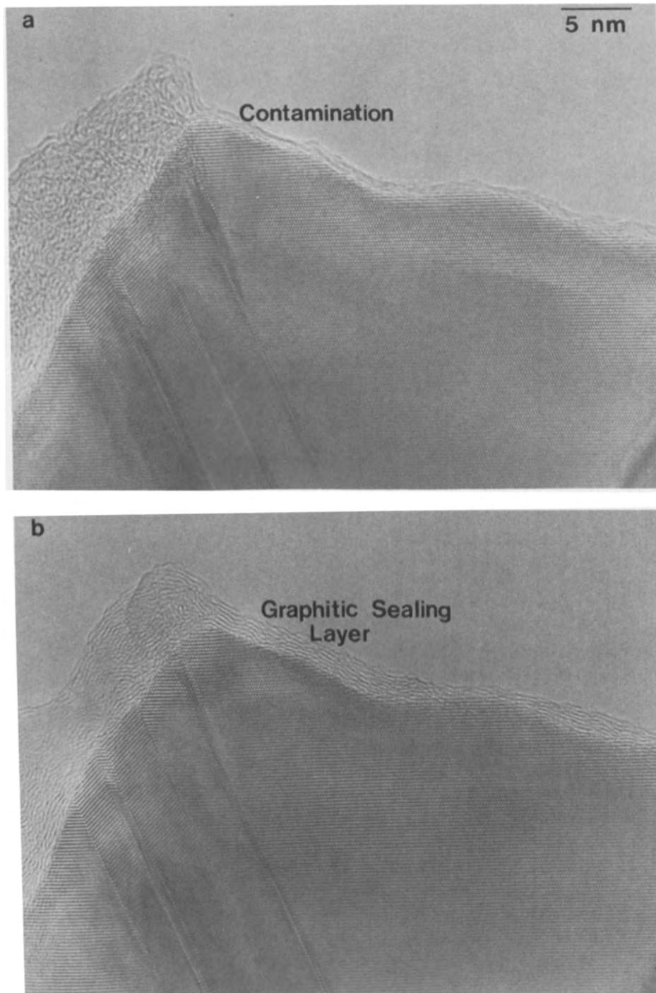
Fig. 2. Series showing damage induced in an encapsulated [111] surface of TiO<sub>2</sub> rutile: (a) initial unirradiated surface, (b) same surface after 2 h irradiation under the 300 kV electron beam.
