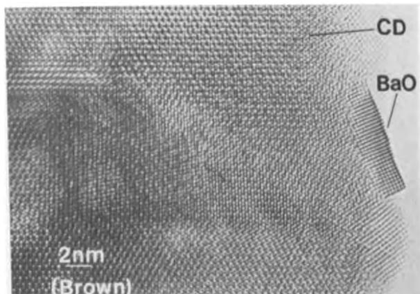
Fig. 3. Under irradiation by the 300 kV electron beam, BaO forms on the surface and chemical disordering takes place in the subsurface region as marked.
