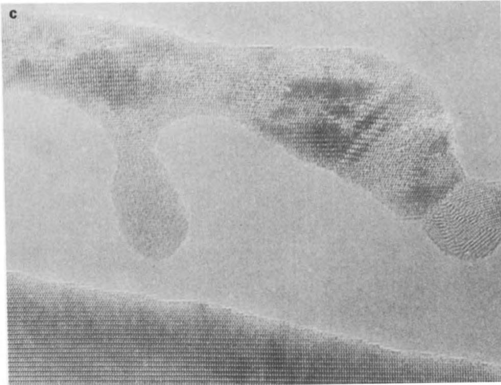
Fig. 1. Series showing damage induced in an unencapsulated [101] surface of  $\text{TiO}_2$  (rutile): (a) initial undamaged surface; (b) a highly defected layer and voids form upon same surface during irradiation; (c) continued irradiation forms a hole due to the coalescence of voids.
