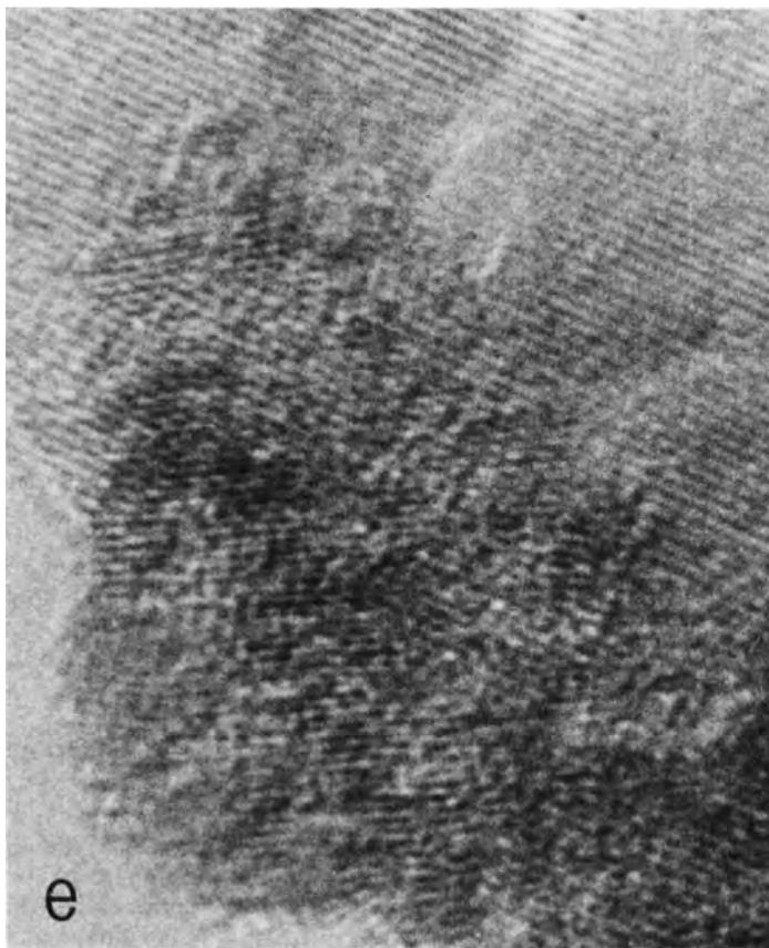
A series of time-lapsed HREM images of  $WO_3$  crystal in  $[100]$  orientation. (a) After 5 min irradiation, inset shows the optical diffractogram from the image. (b) After 20 min irradiation. (c) After 115 min irradiation: inset shows the optical diffractogram from (110) lattice fringes of W. (d) After 160 min irradiation: showing stable critical nucleus of  $WO_3$  crystal. (e) Showing complete disappearance of the  $WO_3$  crystal.
