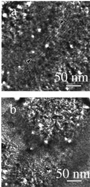
FIG. 1. Dark field image of the Si(001) surface using the Si(220) reflection, (a) prior to ion beam disordering of surface B, nonexposed to direct electron beam during annealing, showing well-ordered steps, (b) after the ion beam roughening, the surface steps are no longer present. Identical bulk defects can be observed in (a) and (b). A step has been arrowed for reference.
