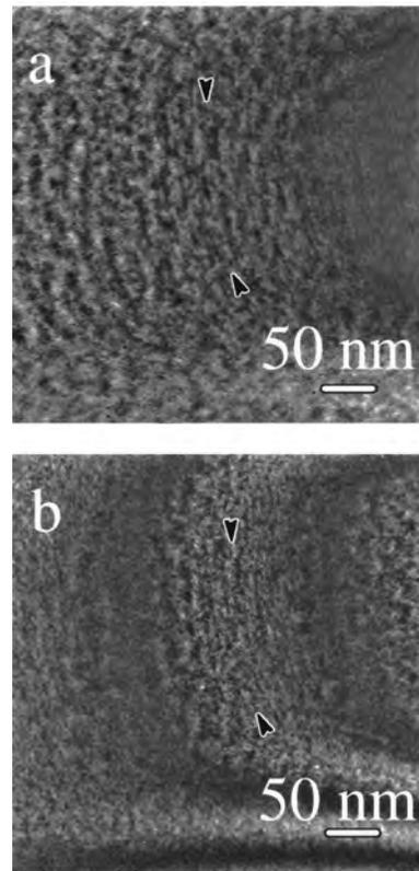
FIG. 2. Dark field image of the Si(001) surface showing the presence of well-ordered steps, (a) prior to and (b) after the ion beam disordering of the sample surface A (incident to electron beam during annealing). A step has been arrowed for reference.
