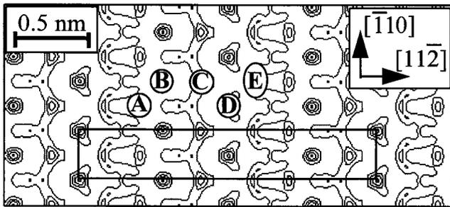
FIG. 3. Contour map of scattering potential found through direct phasing. Peaks A, B, C, and D correspond to Si atoms, and peak E corresponds to two half-occupancy Ag sites. A centered  $6 \times 1$  unit cell is drawn showing the cm symmetry.
