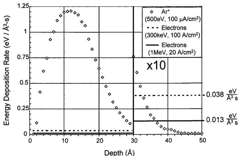
Fig. 1. Rate at which energy is transferred from a flux of ions or electrons to a h-BN crystal through elastic collisions with B or N atoms and recoil energies greater than 20 eV (the h-BN displacement energy). The data for the incident  $\text{Ar}^+$  ions were simulated with amended [14] version of TRIM89 [31] software. The data for the incident electrons were calculated using total displacement cross-sections found with the McKinley and Feshbach [32] approximation to the Mott series [33].
