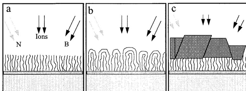
Fig. 7. Depiction of c-BN growth process based on nanoarch nucleation mechanism. (a) Formation of textured t-BN layer. (b) Formation of nanoarches. (c) Cubic BN nucleation and growth.
