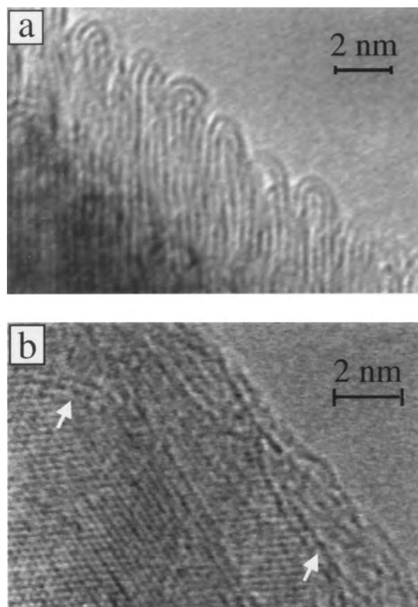
Fig. 3. Same areas that are shown in Fig. 2 after 10-min exposure to 300-keV electron beam with a current density of  $50\text{--}100 \text{ A cm}^{-2}$ . (a) (1120) zone. (b) (0001) zone. Arrows in (b) indicate the arches that are located at the edges of surface steps.
