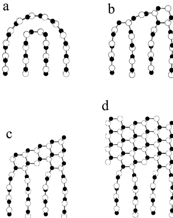
Fig. 6. Conversion of a nanoarch to a c-BN nucleus. The structure in (d) has been shown by Widany et al. [42] to be stable.
