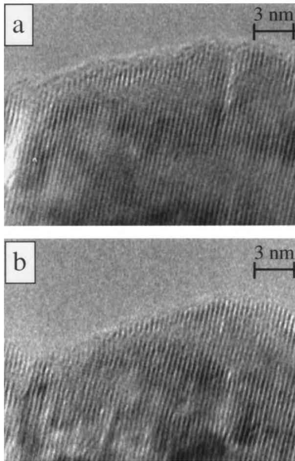
Fig. 5. Images along (1120) zone recorded on H-9000 TEM operating at a vacuum level of  $\sim 5 \times 10^{-7}\text{ Torr}$ . (a) Before electron irradiation. (b) Same region after 10-min exposure to 300-keV electrons at  $50\text{--}100\text{ A cm}^{-2}$  current density.
