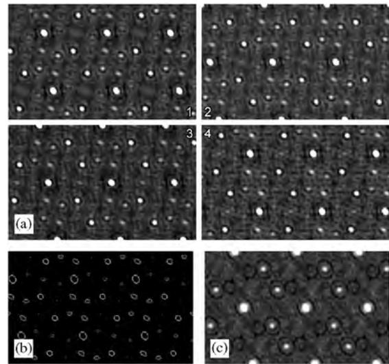
Fig. 5. (a) Four unique DM solutions generated from precession data. Reflections below  $g = 0.25 \text{ \AA}^{-1}$  were excluded. (b) Topographical map of solution 4. Well-defined peaks above the noise floor correspond to atomic positions. (c) DM solution from dynamical dataset. No high-resolution phases were used to generate these maps.
