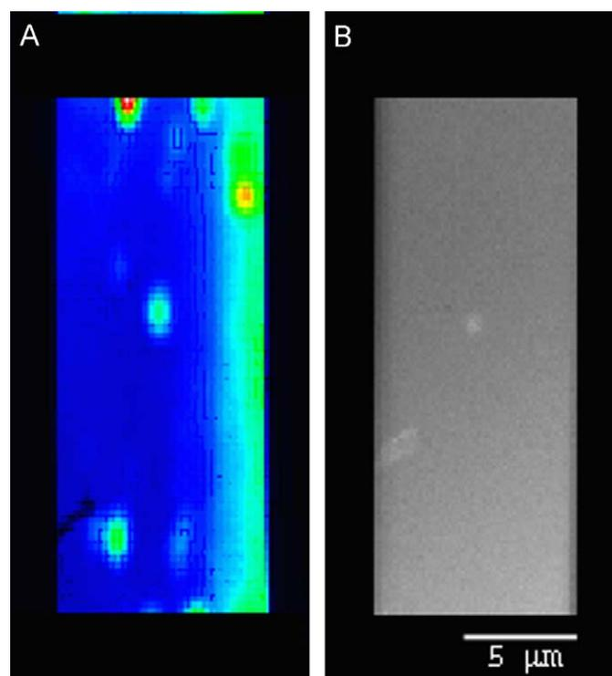
**Fig. 2.** (A) LSPR image and (B) SMSERS image of the same region on the TEM grid.
