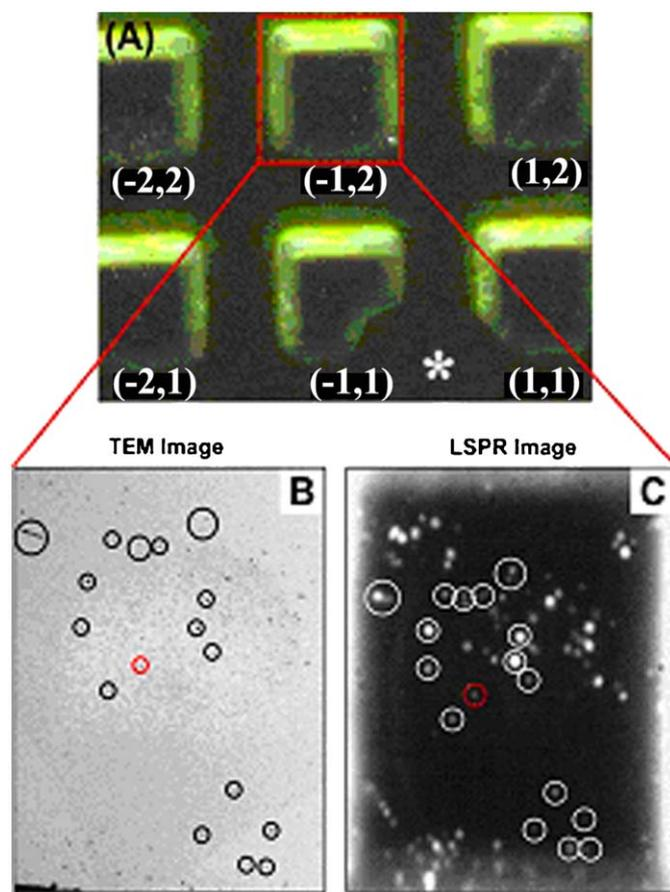
**Fig. 1.** Correlation of TEM and LSPR images. (A) Low resolution ( $40\times$ ) dark-field image of grid (-1,2). Note the distinctive center of the grid in the bottom row, indicated by an asterisk (\*), that can be used as the origin in determining the coordinates, (B) TEM image of grid (-1,2) and (C) LSPR image ( $100\times$ ) of grid (-1,2).
