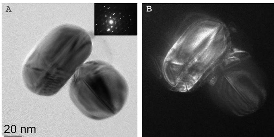
**Fig. 3.** (A) Bright-field with diffraction pattern inset and (B) dark-field TEM image of the SMSERS active nanoparticle identified based on pattern matching using LSPR, SMSERS and low-magnification TEM imaging.
