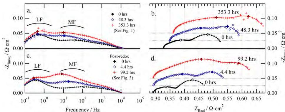
Fig. 2. Bode (a) and Nyquist plots (b) of the impedance spectra recorded at  $t = 0, 48.3,$  and  $353.3 \text{ h}$  during break-in of an LSCrPd–GDC cell. Bode (c) and Nyquist plots (d) recorded after a redox cycle at  $t = 0, 4.4$  and  $99.2 \text{ h}$ . Raw data are presented as symbols and the calculated fits to the spectra are presented as lines. The large diamonds mark the characteristic frequencies calculated from the fits.
