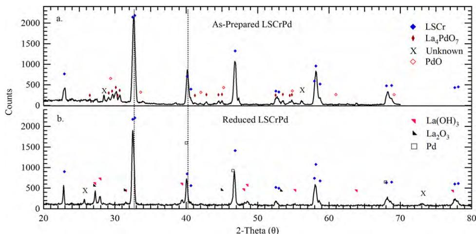
**Fig. 5.** The XRD patterns of (a) as-prepared LSCrPd powder and (b) reduced LSCrPd powder. The symbols show the angle and relative intensities of reflections for various relevant substances, from powder diffraction files.
