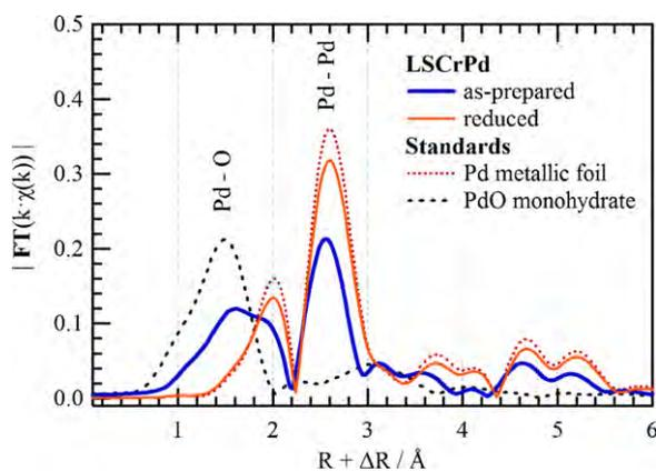
**Fig. 6.** The Fourier transform of the EXAFS for the as-prepared and reduced LSCrPd powder samples and Pd metal and PdO·H<sub>2</sub>O standards.
