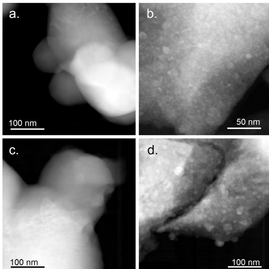
**Fig. 7.** STEM micrographs of LSCrPd (a) as-prepared powder, (b) powder reduced for 1 h at 800 °C, (c) powder reduced for 27 h at 800 °C and then exposed to air for 1 h at 800 °C, and (d) the powder from (c) reduced for 12 h at 800 °C.
