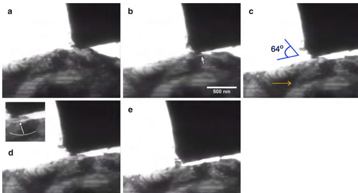
**Fig. 2** Series of TEM micrographs showing chipping of the CoCrMo fcc phase. The attack angle is  $64^\circ$ . A crack is highlighted in the inset figure in (d)
