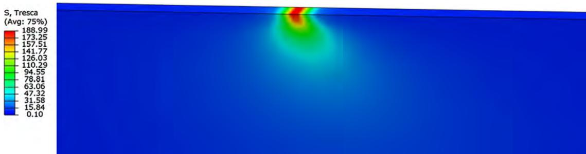
**Fig. 4** Finite element analysis of a simplified thin lamella with a constant applied pressure of 200 MPa on the centre of the top surface. The two sides were fixed. The maximum shear stress is decreased below the contact surface
