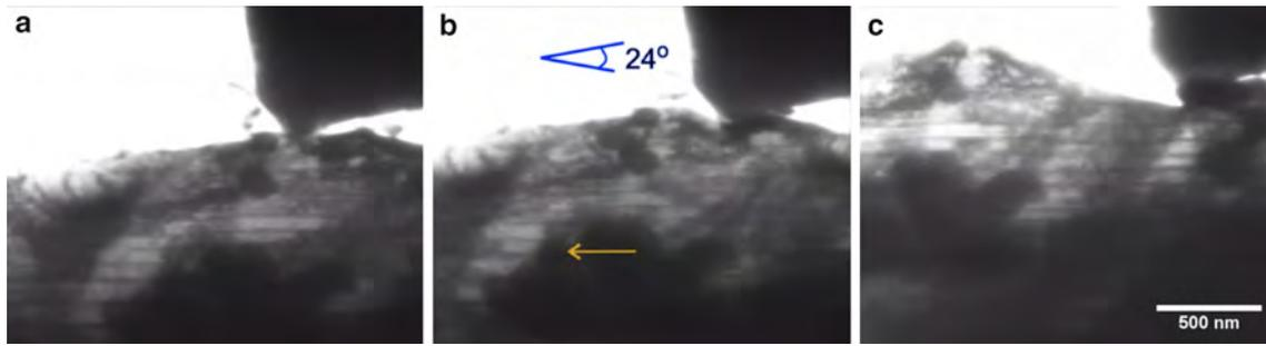
**Fig. 3** Series of TEM micrographs showing wear via ploughing. The CoCrMo thin foil was moving towards the *left*. **a** The initial stage. **b** The tip grooved into the fcc phase. The attack angle is  $\sim 24^\circ$ . **c** Ploughing lasted for 1,160-nm sliding distance, forming an edge ahead of the tip
