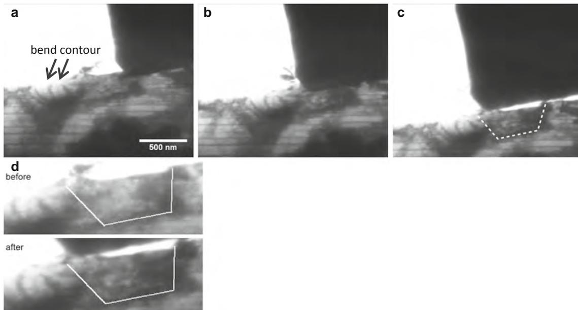
**Fig. 1** a–c Series of TEM micrographs showing plastic deformation in the CoCrMo fcc phase. A dislocation cell is highlighted with the dotted lines. The bend contour arrowed in (a) changed minimally,
