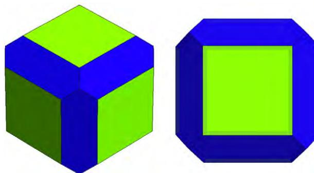
**Fig. 1.** Observed octadecahedral shape of  $\text{SrTiO}_3$  nanoparticles. Note that the coverage of the six  $\{100\}$  facets (green) dominates and thus they are described as nanocuboids. The shape was calculated using the WulffMaker Mathematica code [29] for the  $d_{(110)}:d_{(100)}$  ratio of 1.139.
