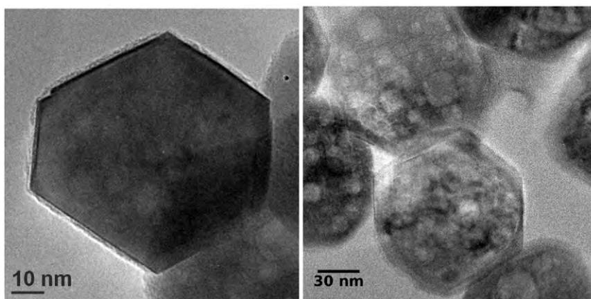
**Fig. 4.** TEM Images of several nanocuboids (also annealed) near [111] zone axis. Note that in both images, the projected shape is hexagonal, indicating that no substantial (111) faceting is present.
