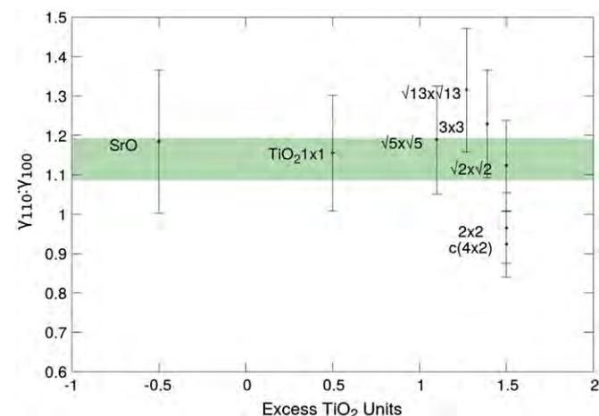
**Fig. 5.**  $\gamma_{(110)}:\gamma_{(100)}$  ratios from first-principles calculations compared within one standard deviation of the mean observed  $d_{(110)}:d_{(100)}$  ratio of 1.139.
