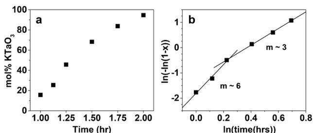
**Figure 2.** (a) Yield of  $\text{KTaO}_3$  in mol % after different lengths of synthesis time. Yield was calculated with Rietveld refinement. (b) Logarithmic plot of the yield showing two linear fits with slopes of  $\sim 6$  and  $\sim 3$ .
