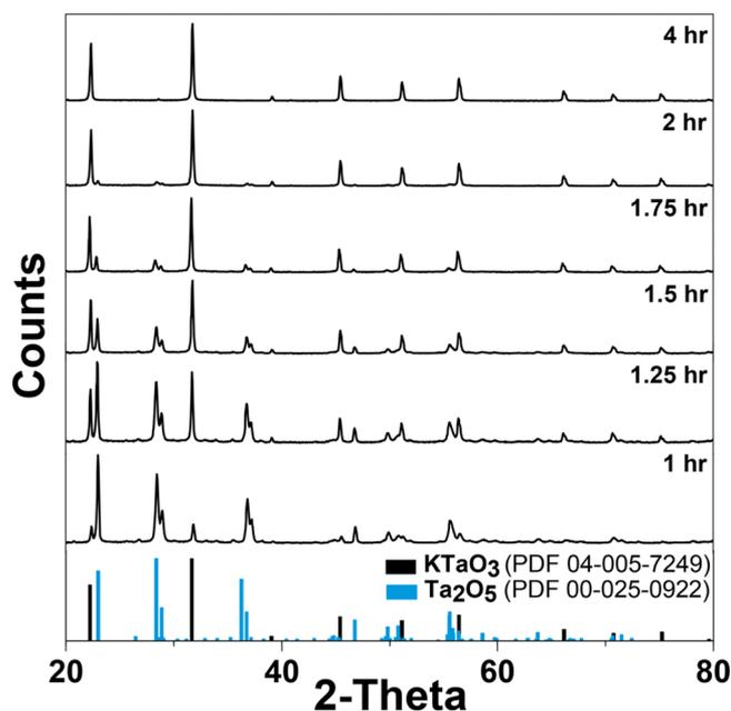
**Figure 1.** XRD patterns of the hydrothermal synthesis products at different time steps between 1 and 4 h of synthesis. Between 1 and 2 h, the patterns show signals from both the reagent  $\text{L-Ta}_2\text{O}_5$  (blue bars, PDF 00-025-0922) and the product  $\text{KTaO}_3$  (black bars, PDF 04-005-7249). At 2 h, the conversion to  $\text{KTaO}_3$  is almost complete, and by 4 h, the product consists of only  $\text{KTaO}_3$ .
