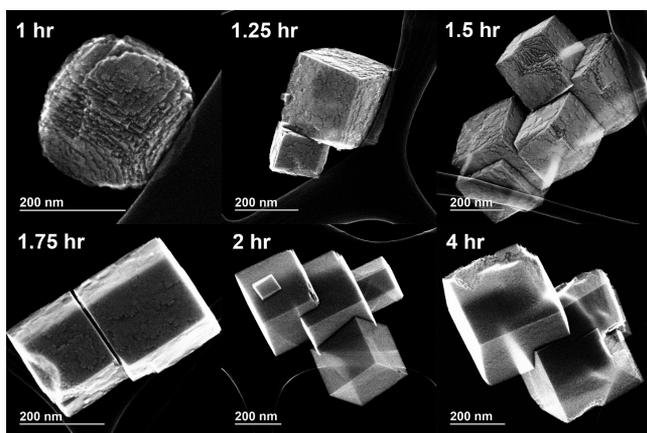
**Figure 3.** SE images of the  $\text{KTaO}_3$  nanoparticles after 1–4 h of hydrothermal synthesis. Images show nanocuboids  $\sim 200$  nm in size with sharp corners and edges.
