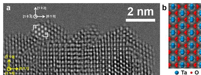
**Figure 5.** (a) Profile-view HRTEM image (with a dose rate of  $30\ \text{e}^-/\text{nm}^2\ \text{s}$ ) of a 4 h  $\text{KTaO}_3$  nanoparticle oriented along the  $[1\ 1\ 0]$  zone with a multislice simulation of  $\text{B-Ta}_2\text{O}_5$  inset (white brackets). (b) Image simulation of  $\text{B-Ta}_2\text{O}_5$  with the atomic structure superimposed, where large blue atoms are Ta and small red atoms are O.
