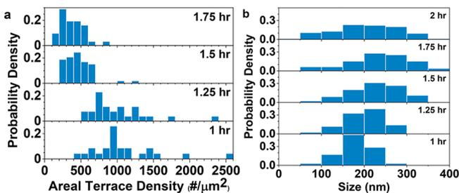
**Figure 4.** (a) Histogram of areal terrace density measured on nanoparticle facets for 1, 1.25, 1.5, and 1.75 h hydrothermal synthesis products. Histograms show narrowing distributions and decreasing densities with time. (b) Nanoparticle size distribution for synthesis times between 1 and 2 h. Distributions broaden with increasing time, and the average size increases with increasing time until 2 h, where the average size begins to decrease. (See enlarged plots in Figure S2.)
