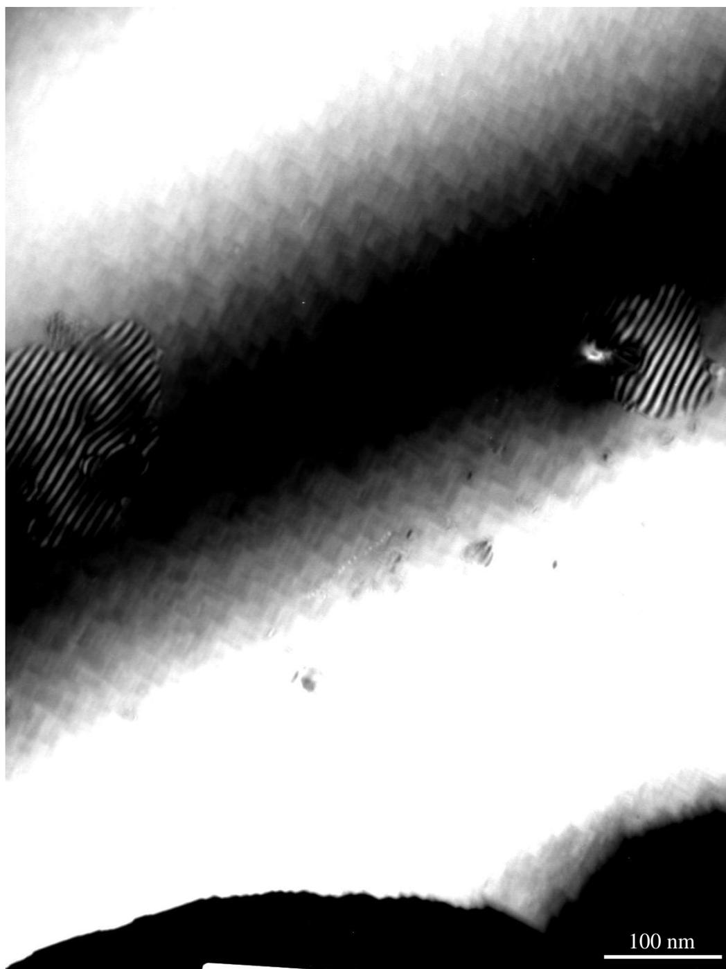
**Figure 4.13:** Dark-field TEM image showing  $\text{TiO}_2$  particles growing on the surface of  $\text{SrTiO}_3$ .
