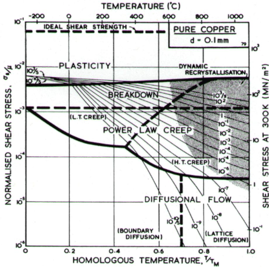
Figure 6.2: Deformation mechanisms map for copper, showing the temperatures and stresses where power law creep dominates. [130]
