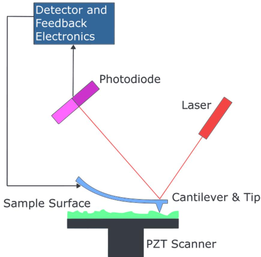
Figure 3.1. Typical schematic of an AFM courtesy of Wikipedia. The tip is rastered along the surface and a 2D image is usually created from either the changing z-position of the tip or the force necessary to maintain a constant height. Other modes are available as well.
