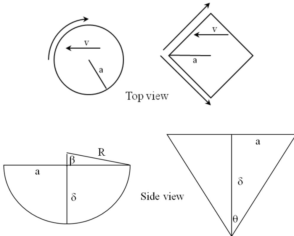
Figure 6.3. Top: The top view of (left) spherical and conic asperities and (right) square pyramidal asperities as they plow through material. The arrows show the distance the plowed material has to travel whenever the asperity advances by one radius. The contact radius  $a$  actually cancels out resulting in the same strain rate regardless of size.
