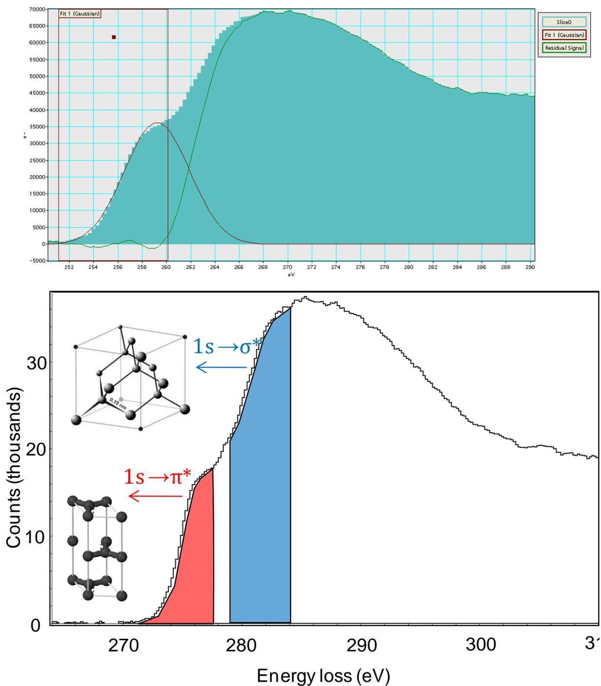
Figure 4.2. Top: Experimental EELS spectrum showing Gaussian fitting in order to calculate  $sp^2$  and  $sp^3$  signals. Small amounts of energy shift tend to occur over time, and are taken into account during the analysis of sequential spectra. The energy loss is also calibrated before each sliding test. Bottom: Experimental EELS spectrum showing how count integration is done and different electron transitions correlated with  $sp^2$  or  $sp^3$  carbon bonding.
