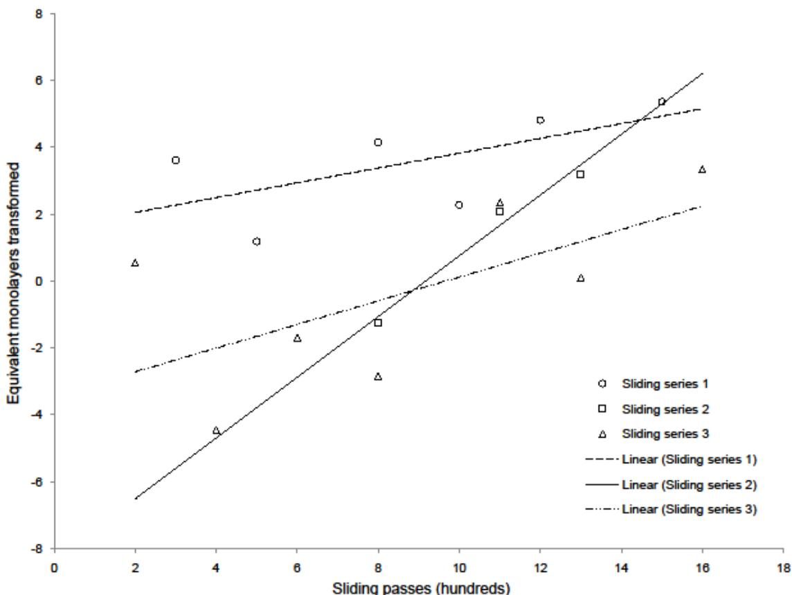
Figure 4.4. Trendlines of equivalent monolayers transformed for three sliding series. The data points show the equivalent number of monolayers transformed from  $sp^3$  to  $sp^2$  bonding. Negative values represent a transformation in the opposite direction, something which is attributed to drift and other factors near the beginning of the sliding experiment. A trendline is shown for the data points measured relative to the initial condition.
