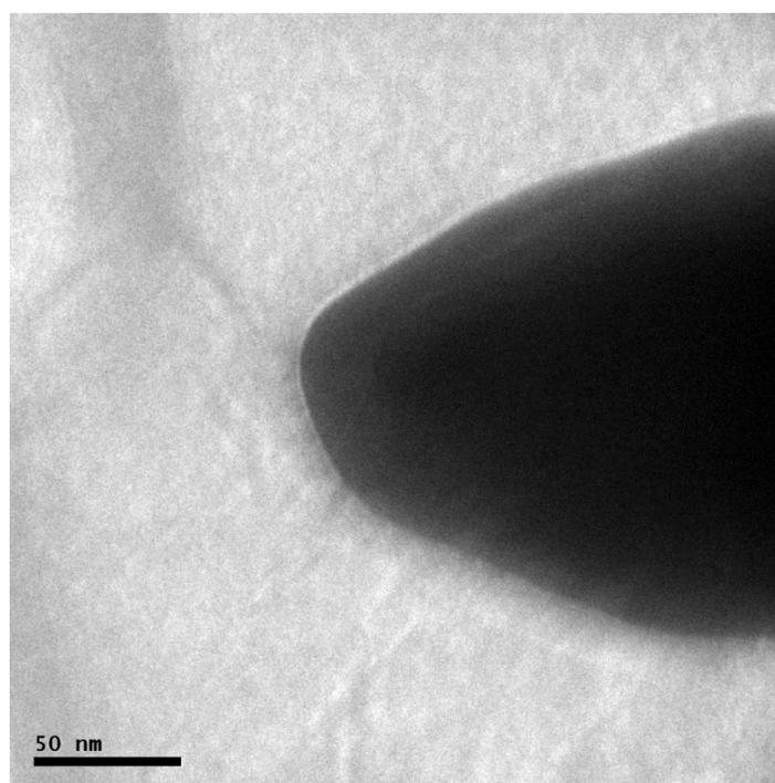
Figure 3.8. TEM micrograph of a typical tungsten probe tip prepared by electrochemical etching.
