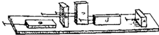
Figure 1.2. Sketches from the Codex Atlanticus and Codex Arundel showing Leonardo da Vinci's studies of the contact area dependence of friction. [1]
