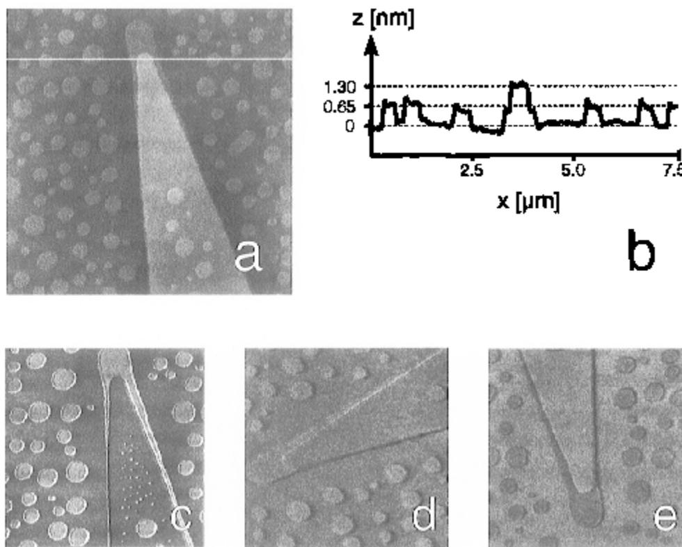
Figure 3.2. Triglycine sulfate studied with lateral force microscopy. (a) is a  $7.5 \mu\text{m}^2$  topography map while (c), (d), and (e) show friction force scans of the same area at different orientations, highlighting the dependence of friction on the details and directionality of the crystal. [32]
