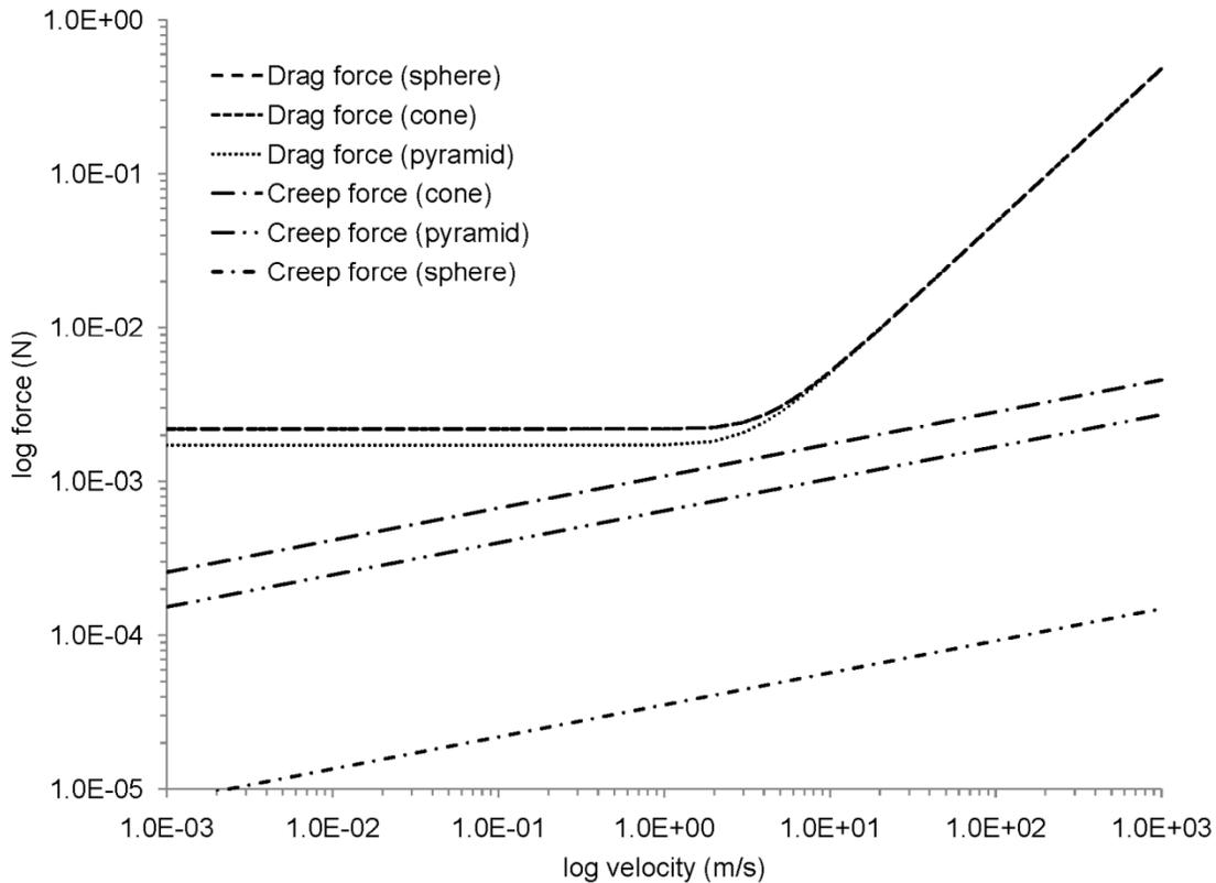
Figure 6.5. Creep and drag forces vs. sliding velocity and asperity shape. Normal load 10 mN, temperature  $0.8 T_m$ , cone/pyramid angle  $20^\circ$ , and sphere radius of curvature  $1 \mu\text{m}$ .
