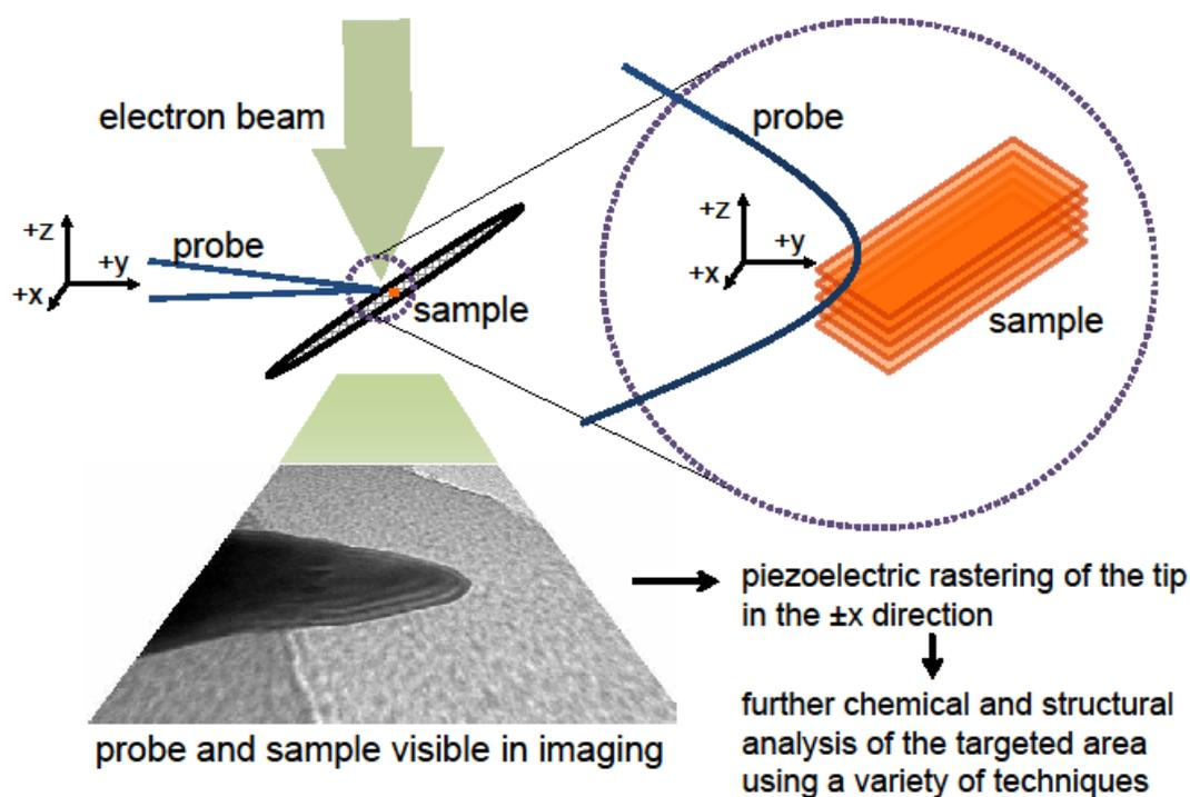
Figure 3.3. Schematic of the Nanofactory HS-100 STM-TEM holder inside the microscope column. The TEM micrograph shown represents a typical view of the probe tip inside the microscope column. The motion directions available to the tip are labeled  $x$ ,  $y$ , and  $z$ , and are not absolute coordinates. The sample itself is mounted in a full-size TEM grid rotated  $45^\circ$  about the  $x$ -axis as shown, and the sliding is typically done in the  $\pm x$  direction.
