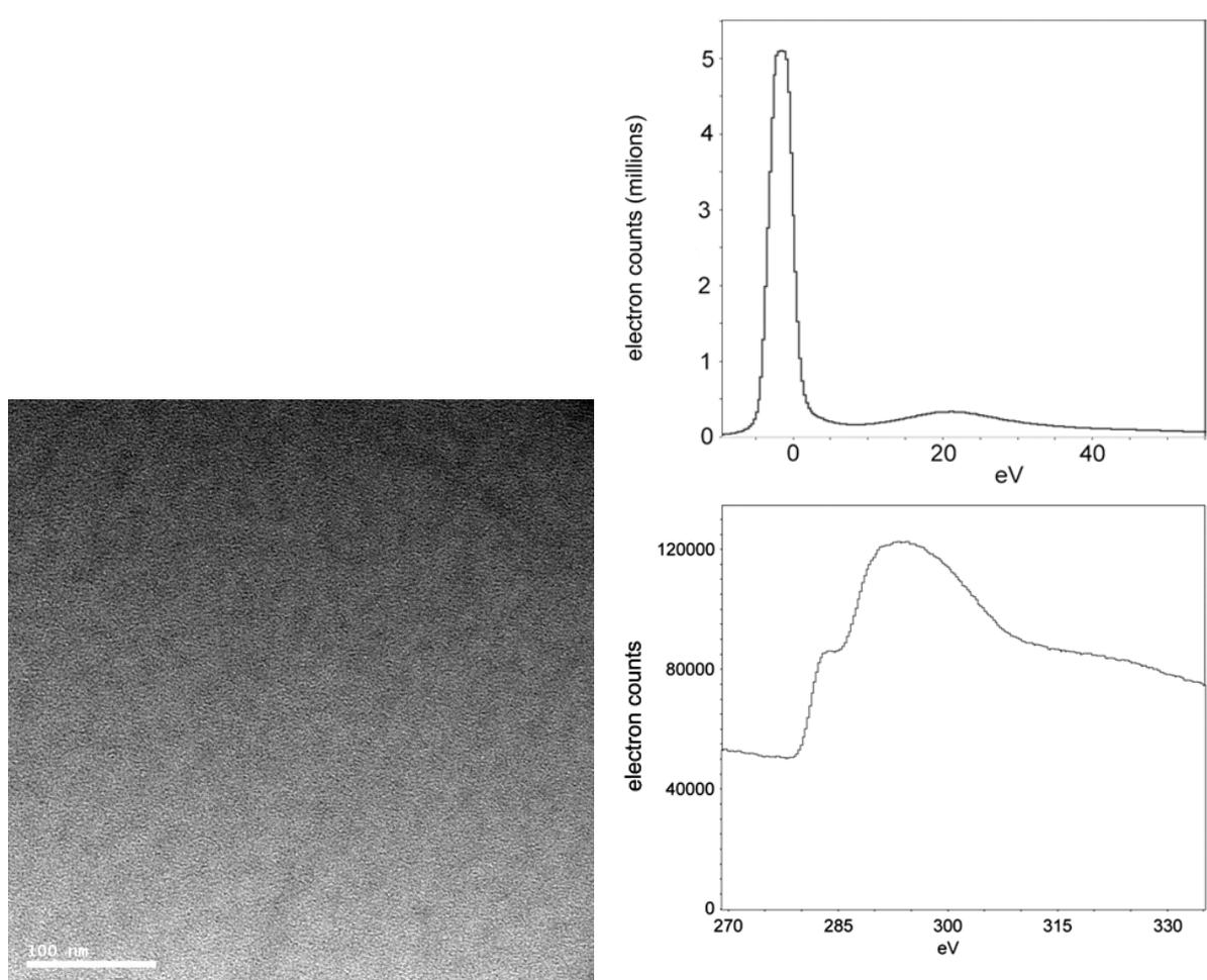
Figure 4.1. Left: DLC film bright field electron micrograph from a pristine region of the sample. Right: Zero-loss and carbon K-edge EELS spectra from the same area.
