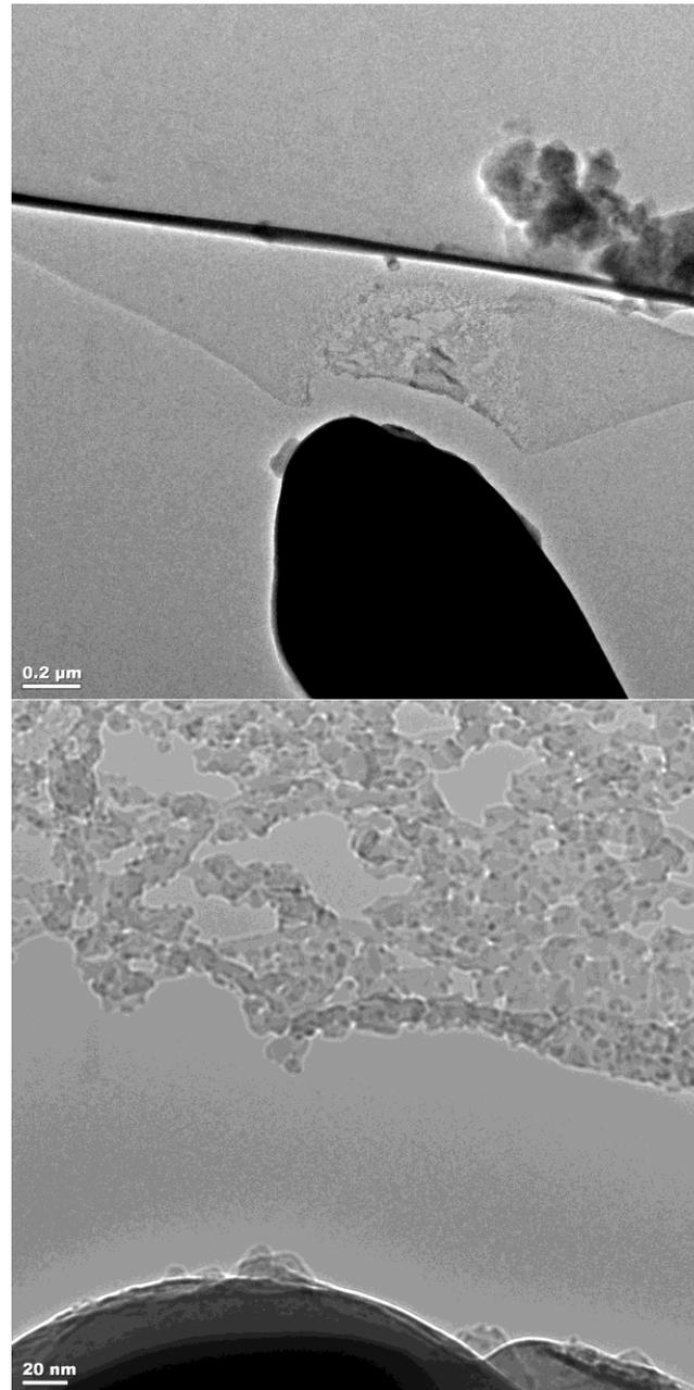
Figure 5.7. TEM micrographs showing DLC film damage after long term exposure under the electron beam. In higher gas pressures, the general etching of the films occurred faster.
