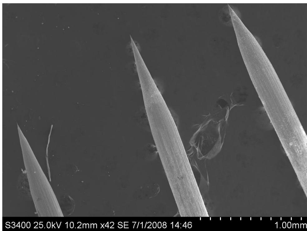
Figure 3.7. SEM image of prepared tungsten probes showing the desired tip aspect ratio.
