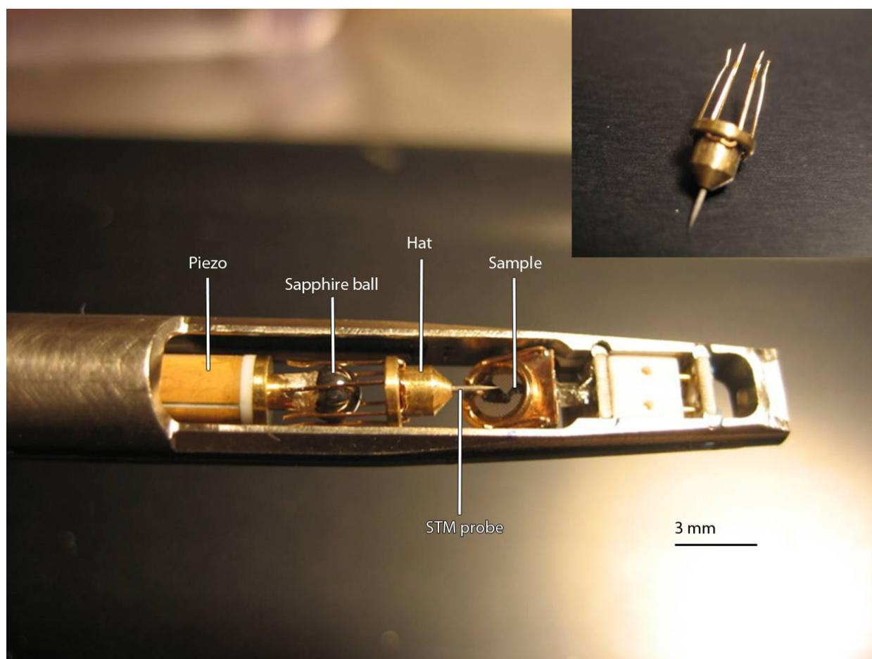
Figure 3.4. Photograph of the tip of the Nanofactory HS-100 STM-TEM sample holder. Shown are the mounted sample, probe, and control mechanisms: piezoelectric tube and a rotatable sapphire ball pulsed for coarse stick-slip motion.
