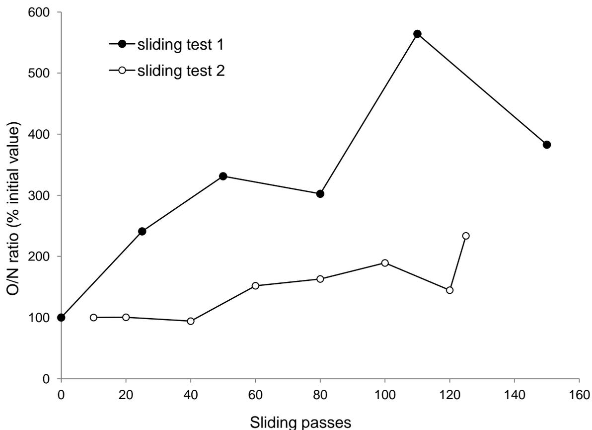
Figure 5.4. The ratio of oxygen to nitrogen edge counts is measured using EELS to increase over the course of the sliding experiments in wet  $N_2$ . The percentage increase of the ratio of the signal reflects the actual proportional change in bonding in the sampled area. The EELS counting process has negligible error, although there are systematic errors associated with sample drift, etc. The increasing O/N ratio suggests incorporation of oxygen into the solid phase during sliding.
