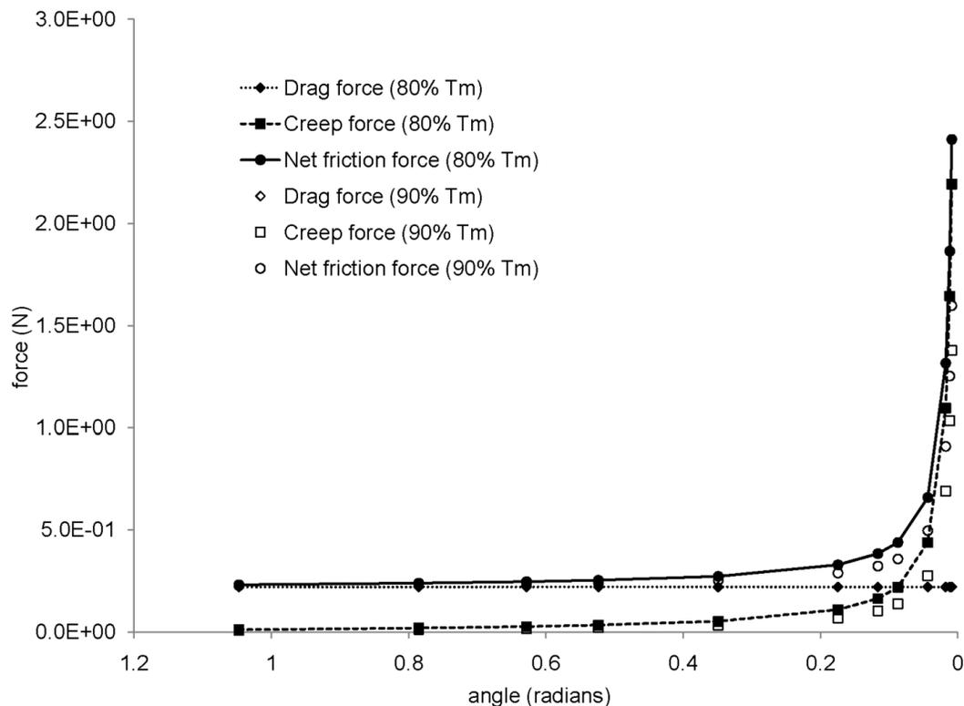
Figure 6.6. Friction force vs. cone angle and temperature. For a cone-shaped asperity, 1 m/s, 1 N load. A decrease in the cone angle corresponds directly to an increase in the penetration depth of the asperity, for the same normal load.
