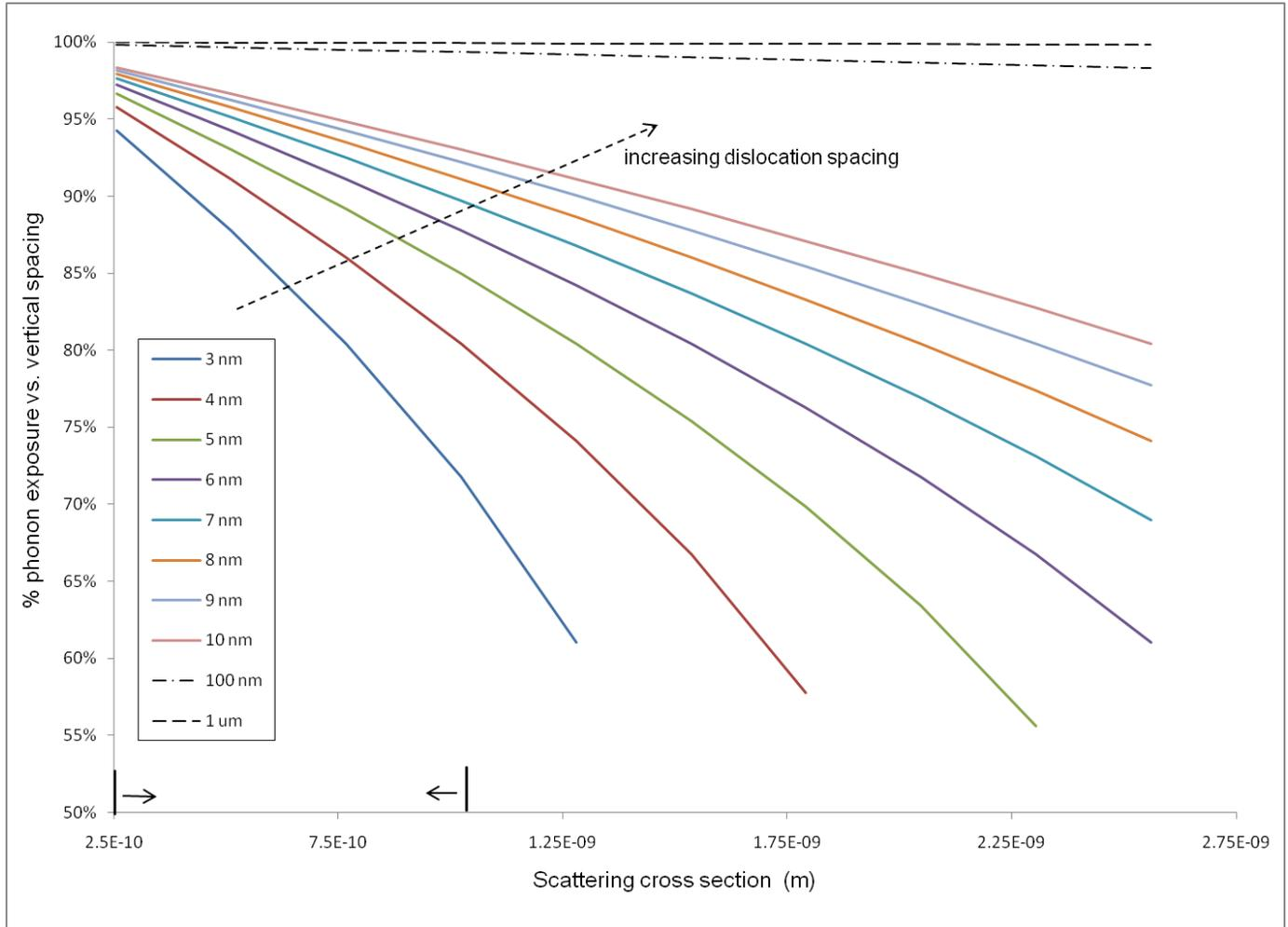
Figure 7.2. The percentage of phonons that will be incident on the shielded dislocation, as a function of scattering cross-section – 100% represents no shielding effect, 0% represents complete shielding. Results for a range of spacings are shown. The relevant cross-sections are indicated with bounding arrows, encompassing the range between one-half and twice the average  $\sigma = 2b$ .
