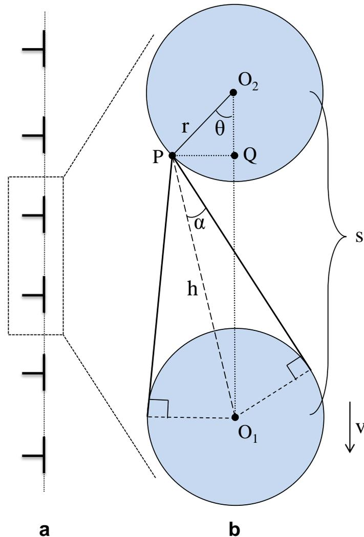
Figure 7.1. Schematic of the shielding geometry. **a)** A typical array of edge dislocations with the same Burgers vector glide through a crystal on a slip plane. Phonons incident on the array with momentum counter the direction of motion are considered. **b)** Nearest neighbor dislocations in a 1-D array are represented as spheres, and reduced here to circles due to spherical symmetry.
