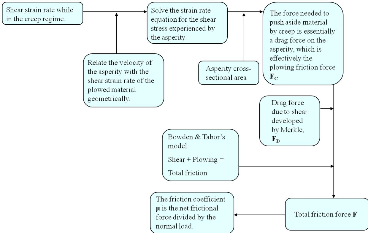
Figure 6.1. Flowchart of the analytical friction model.
