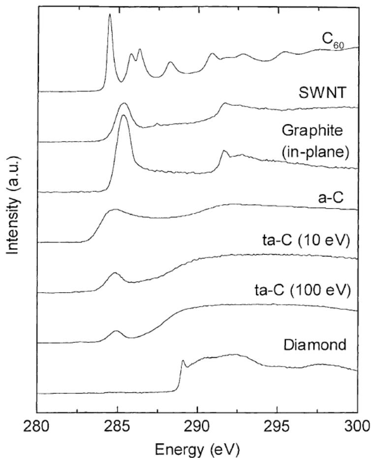
Figure 3.9. EELS carbon K-edge spectra for various forms of carbon, as seen in [62].
