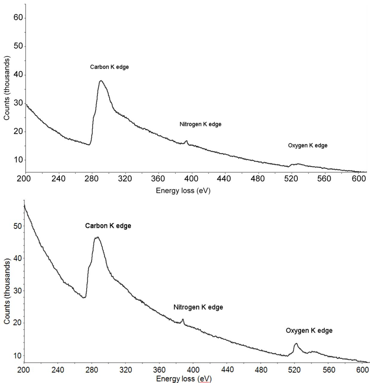
Figure 5.3. EELS spectrum after 0 (top) and 110 (bottom) sliding passes in wet  $N_2$  showing the relative prevalence of chemisorbed oxygen to nitrogen. Quantification suggests a two- to four-fold increase in the relative amount of oxygen compared to nitrogen present in the sampled volume over the course of a sliding experiment.
