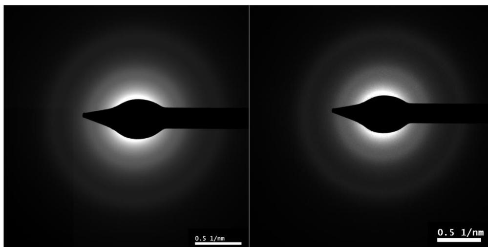
Figure 4.5: Nanodiffraction patterns of the same region of film before (left) and after (right) a sliding experiment. The approximate sample area is 800 nm in diameter.
