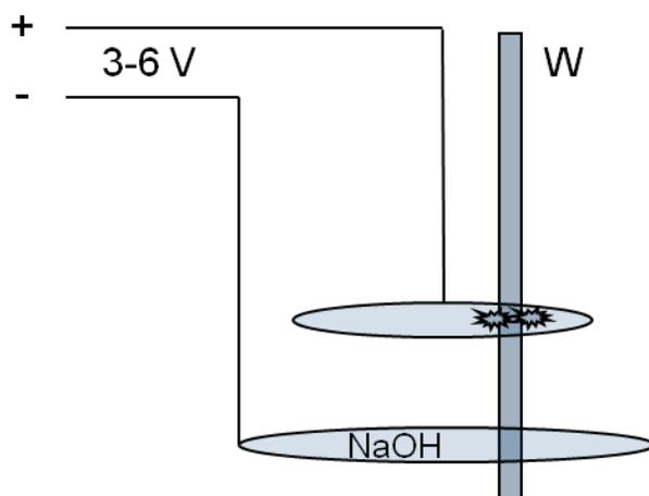
Figure 3.6. Schematic of the electrochemical etching (electropolishing) apparatus. The NaOH solution is held in tension inside loops of gold wire. With an applied bias, etching takes place in the meniscus formed about the vertically placed tungsten wire. When the wire is etched through, the circuit is broken and etching ceases. Both halves of the wire often have usable sharp tips.
