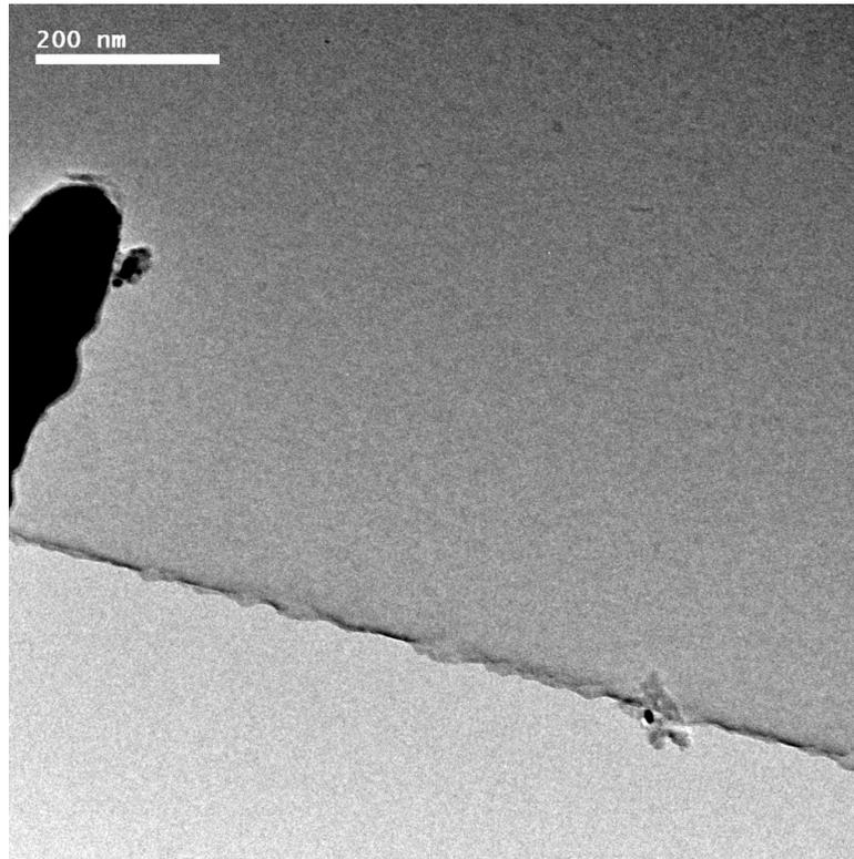
Figure 5.6. Bright field TEM micrograph of a DLC film after the conclusion of a sliding experiment in vacuum. No significant wear tracks are observed in these experiments.
