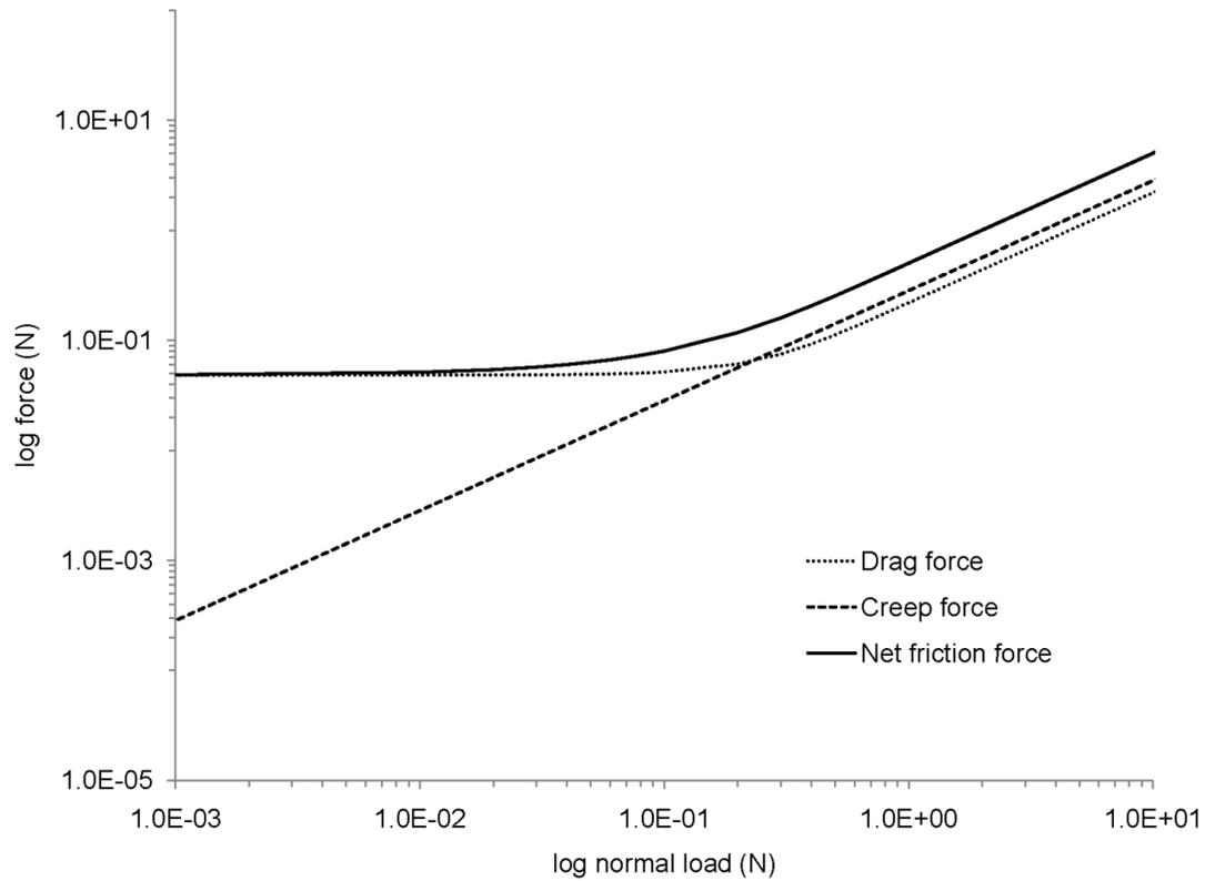
Figure 6.4. Friction force vs. normal load. 100 m/s sliding velocity, and cone angle 10°.
