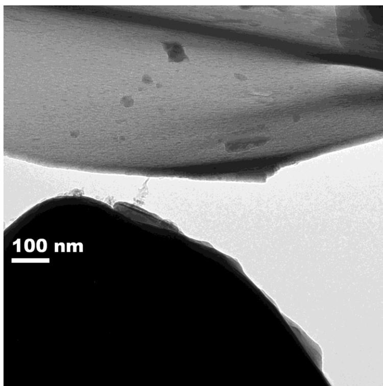
Figure 5.5. Bright field TEM micrograph at the conclusion of a wet H<sub>2</sub> sliding experiment. No significant wear tracks are observed at the conclusion of the test, which used the same type of contact and sliding speed as previous tests. Some light markings and wear particles are visible at the end of the test, but not at the scale as N<sub>2</sub> experiments.
