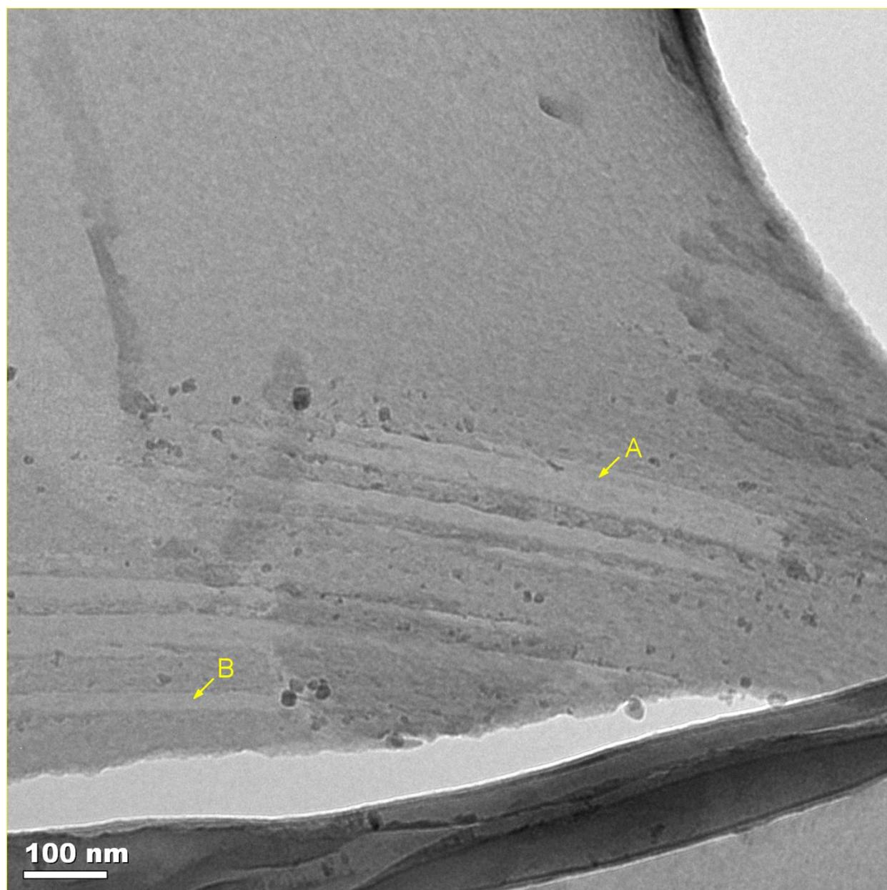
Figure 5.1. Energy filtered (zero-loss) TEM micrograph showing the surface of a 26 nm thick DLC film during a wet N<sub>2</sub> sliding experiment after 20 sliding passes. Arrows indicate lighter regions, which are interpreted as thinner due to the amorphous nature of the film. As A and B have different background brightness levels, separate calculations were done in each part of the micrograph in order to determine the estimated volume lost.
