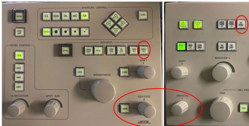
11. Objective stigmatism: acquire an image of amorphous region (>500 kx) in GMS3 (Gatan PC, middle) using RIO camera. You need to insert the camera first. Click Process >> Live >> FFT, press **OBJ STIG** and adjust **DEF-X** & **DEF-Y** knobs to make the FFT pattern round.
