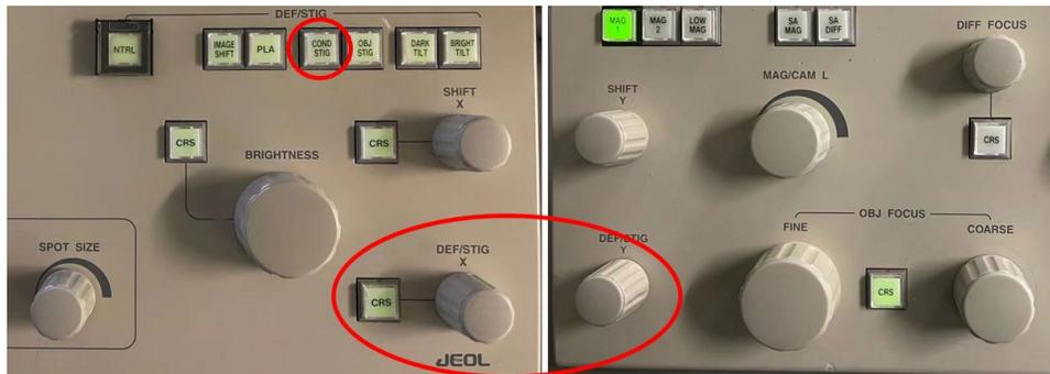
7. Check/Align Gun Tilt: at 40kx, press **F3** “Anode Wobbler”, press **F4** “GUN Align”, adjust **DEFLECTOR-X** & **DEFLECTOR-Y** knobs to get a uniformly expanded beam.
