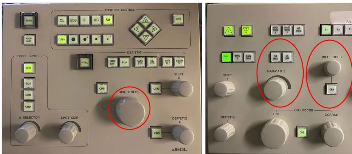
2. Insert selected area aperture: press **SA** and desired size number (left panel). You need to align the selected aperture well with the beam by clicking the UP/DOWN/LEFT/RIGHT arrows.
