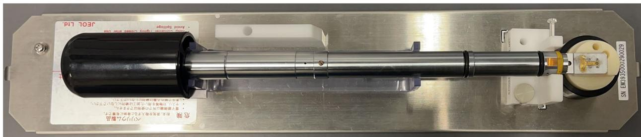
3. For single tilt holder, loosen two screws TWO turns, rotate the cover plate away and mount specimen with film side UP.
