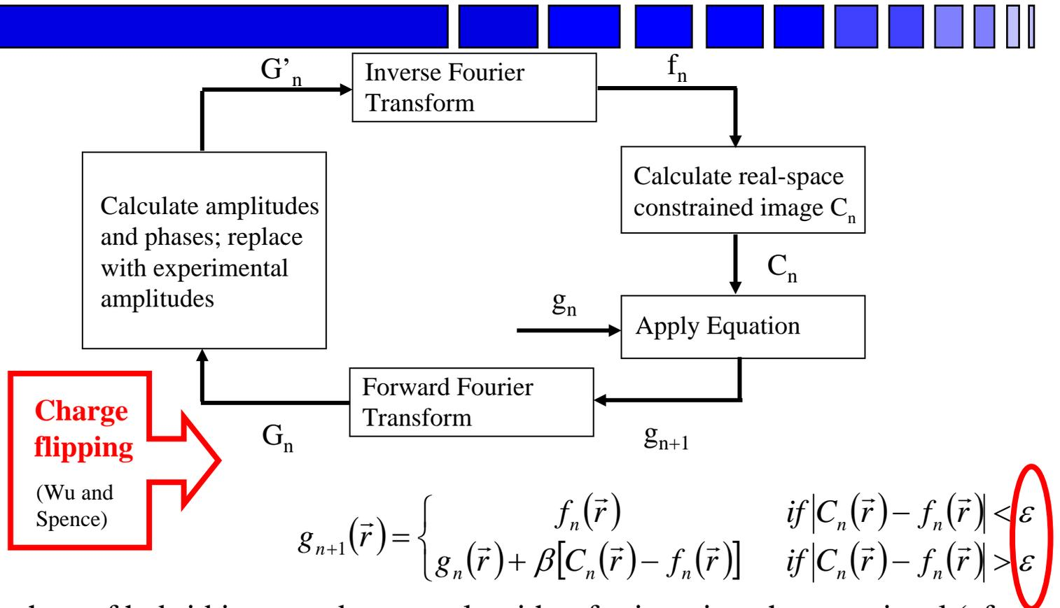
The flow chart of hybrid input and output algorithm for iterative phase retrieval (after Millane and Stroud, 1997).
