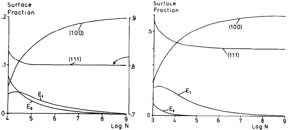
Fig. 2. Plot of the surface fraction of (111), (100) and edge atoms  $E_1$  and  $E_2$  as a function of  $N$  for an equilibrated broken bond (BB) model. The curve for the (111) atoms is drawn using the scale to the right. The strong drop in the fraction of (100) surface should be noted. We note that the sum of (100) and  $E_1$  atoms is essentially a constant fraction.
