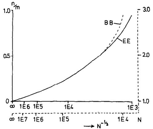
Fig. 5. Plot of  $n/m$  for the equal energy (EE) model against  $N^{-1/3}$  - the solid curve and axes. For comparison,  $n/m$  against  $(N/2)^{-1/3}$  for the broken bond (BB) model is shown by the dashed curve and axes. Except for small clusters, the two curves are identical.
