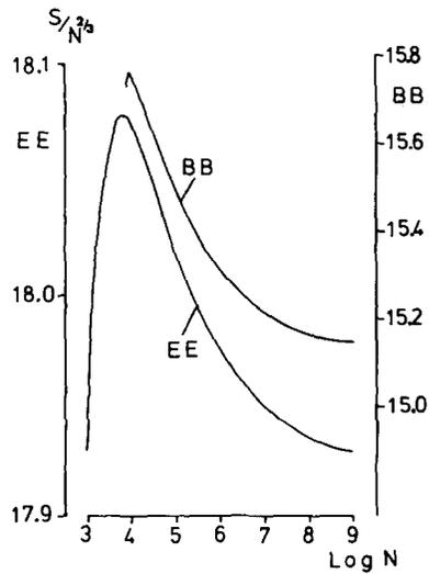
Fig. 7. Variation of  $S/N^{2/3}$  against  $N$  for the broken bond (BB) model, axis shown to the right, and equal energy (EE) model for which the axis is shown on the left.
