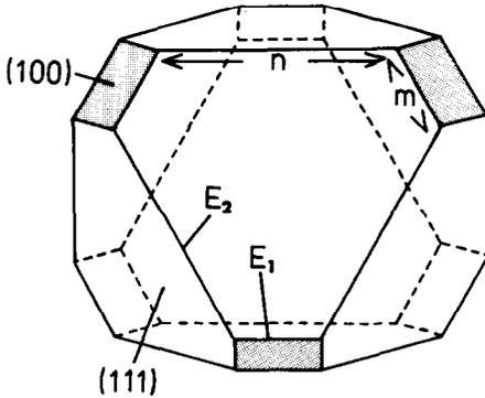
Fig. 1. Diagram of the simplified fcc particle used in the analysis, showing the definition of  $n$ ,  $m$  and the edges  $E_1$  and  $E_2$ . Note that  $n$  and  $m$  correspond to the number of atoms along the edges  $E_2$  and  $E_1$  respectively, which scale to the lengths.
