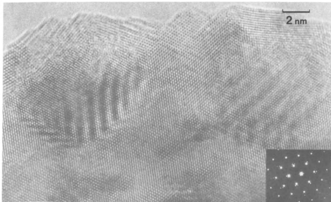
Fig. 6. A “dirty” NiO sample irradiated under low flux conditions at 300 kV for 0.25 h. Islands of Ni have formed on the surface with a cube–cube epitaxial relationship.
