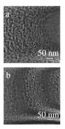
FIG. 1. Dark field image of the Si(001) surface using the Si(220) reflection, (a) prior to ion beam disordering of surface B, nonexposed to direct electron beam during annealing, showing well-ordered steps, (b) after the ion beam roughening, the surface steps are no longer present. Identical bulk defects can be observed in (a) and (b). A step has been arrowed for reference.
