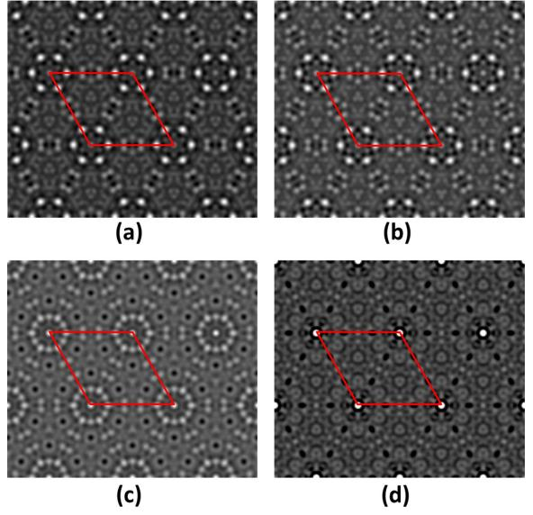
**Fig. 4.** Simulated HREM images of the  $(3 \times 3)$  surface reconstruction on SrTiO<sub>3</sub> (111) after bulk removal at varying thicknesses in (a) 5 nm, (b) 6.33 nm, (c) 7.7 nm and (d) 9.07 nm. (The  $(3 \times 3)$  surface unit cell is outlined in red.). (For interpretation of the references to color in this figure legend, the reader is referred to the web version of this article.)
