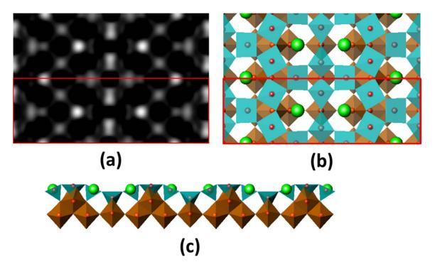
**Fig. 1.** In (a) experimental image of the  $c(6 \times 2)$  surface reconstruction after the removal of bulk and separation of top and bottom surface from high resolution plan view transmission electron microscopy image and the corresponding structure in (b) plan view and (c) profile view. (The unit cell is outlined in red.). (For interpretation of the references to color in this figure legend, the reader is referred to the web version of this article.)
