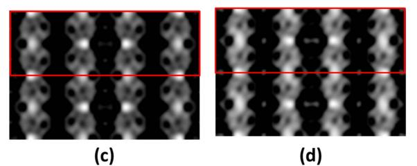
**Fig. 2.** Simulated plan view images after bulk removal (defocus = 6 Å) at thicknesses of (a) 4.15 nm, (b) 5.32 nm, (c) 6.49 nm and (d) 7.66 nm. Vibration of 0.4 Å (root mean squared) in the *x*- and *y*-directions has been added to all images to mimic experimental conditions. (The  $c(6 \times 2)$  unit cell is outlined.).
